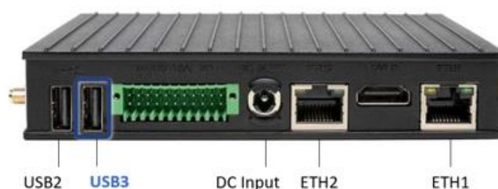
Figure 9: Horizon Power's SGD hardware and port overview 1
